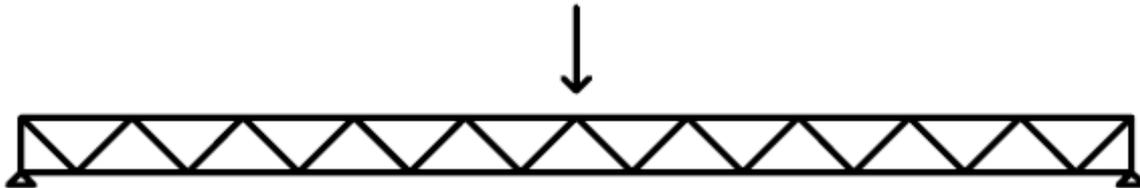
LF 3: Einzellast in den Drittelpunkten, symmetrisch angeordnet in den Knoten der Unter- oder Obergurte. / *Point loads in the third-points, symmetric on bottom or top tubes in the intersection of vertical braces with the main tube.*
