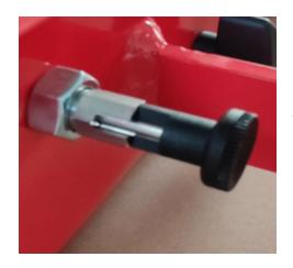
In the first step, both the locking bolts and the screws are unscrewed so that they do not interfere with inserting the adapter.
