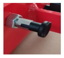
In the second step insert the forklifter adapter into the dolly from above, bevel the holder slightly and pay attention to the fixing holes in the dolly frame when positioning. If the forklifter adapter is roughly positioned, the locking bolts can be turned to their original position. If necessary move the holder back and forth a little until all bolts have snapped into place. Then tighten the screws.
